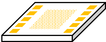
ROIC with planarized contacts
